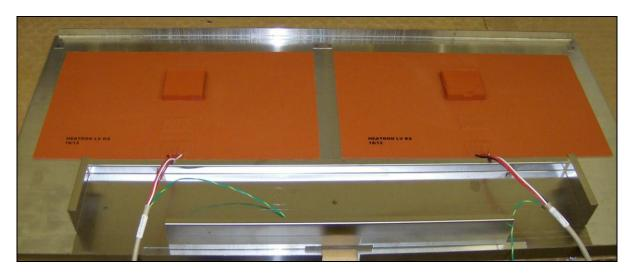
**Step 14:** Reassemble and reinstall the heater shelf (reverse of steps #10 through #13). Reconnect the heater cable.
