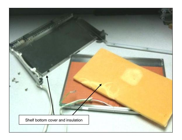
**Step 6:** Peel the failed heater off of the bottom of the shelf.
