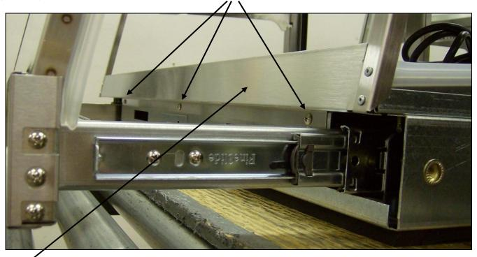
This frame can be pulled forward to allow removal of the lower hot plate.
