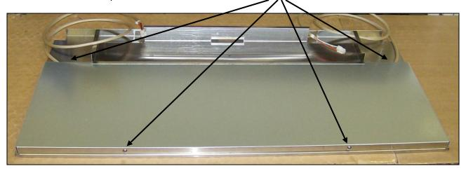
Step 13: Remove the cover and insulation. Replace the heater element as described in Steps 6 and 7.
