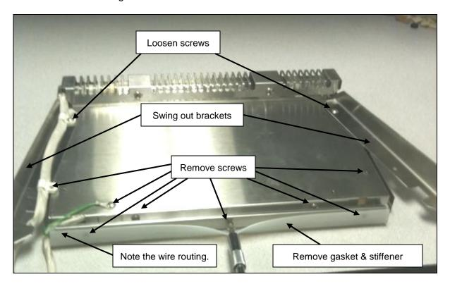
**Step 5:** Remove the shelf bottom cover and insulation.
