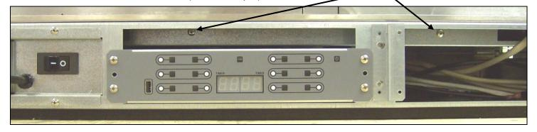
**Step 11:** Open the front of the HFD and remove these three screws.
