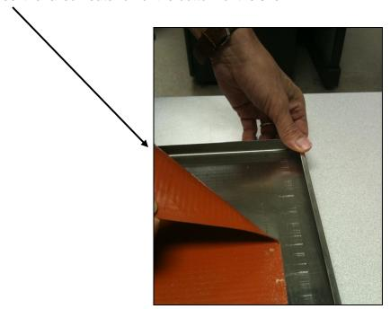
**Step 7:** Remove the release liner from **1201358 Heater**, **HFD** (supplied with this kit). Position the heater on the shelf in the same position as the old heater. Apply the heater starting at an edge and insure there are no air bubbles larger than 0.1 inch diameter or wrinkles. Insure <u>all areas</u> of the heater have been firmly pressed against the hot plate, including the features protruding from the heater. Route the wires as they were before.
