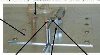
Push units together and add  $\underline{V802291}$  Bolt, 2 ea  $\underline{V801491}$  washer and  $\underline{V800898}$  nut. Remove lower deck panels.
