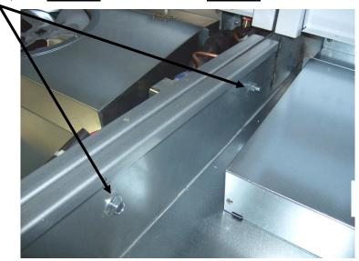
Tighten all 3 nut and bolt sets. Reinstall lower deck panels.
