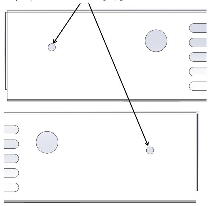
**Step 4:** Reinstall panel and install screws in holes that were added to panel.
