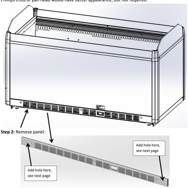
**Step 3:** Drill two ¼ inch diameter holes in locations shown. The images below are full size when printed, so the location can be marked using this page.
