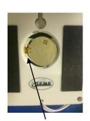
Insert left side of battery below pins
