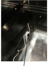
Run wire down the back of the case into the drain pan.
