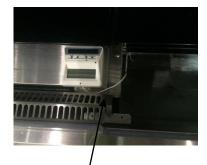
Run wire through channel and place the thermometer all the way forward by the grill so the solar panel has access to light.
