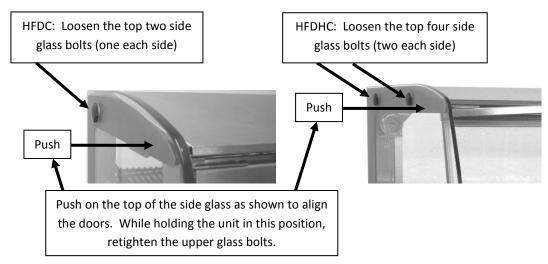
Note: shown above is the left door higher than the right door. Mirror this procedure if the right door is higher than the left door.
