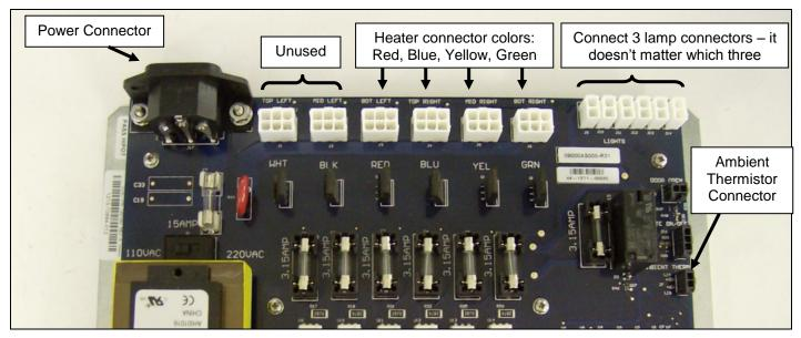
Step 9: Push the cables and controller into the HFD base and reinstall the screws holding the controller.
