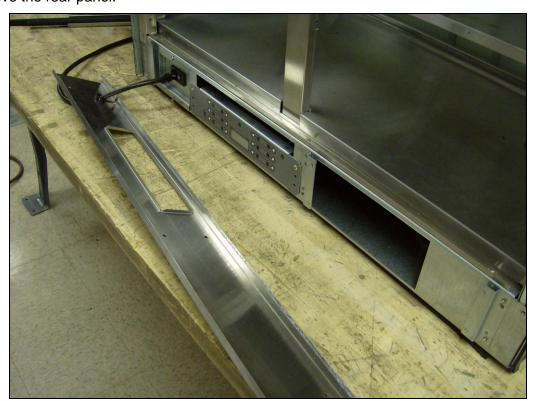
**Step 3:** Remove the screws holding the breaker panel and controller. Disconnect and remove the controller. Pull out the breaker panel.
