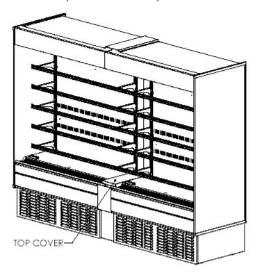
**Step #14** Place glass shelves and rear shelf supports on each shelf. The rear shelf support is placed against the back edge of the glass.
