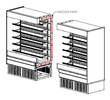
**Step #5** Push the two units together. Install the (7x) 3/8" bolts, washers and nuts in the extentions but do not tighten. There are 2 bolts in the top and bottom and 3 along the back. Using 9/16" socket wrench and cresent wrench, first attach the upper extension. You will need to use a small stepladder to reach the top two bolts.
