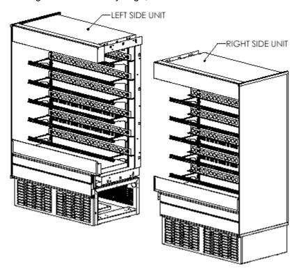
Step #4 While units are apart, place silicone along the lower, back and upper extension parts as shown.
