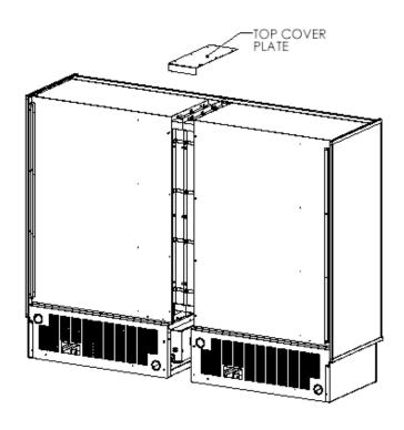
Step #9 Install rear foam blocks and upper back plate cover by placing the oblong cutouts around the screw heads and using (6x) black self-tapping screws (p/n V801489) in the bottom 6 holes to secure it.
