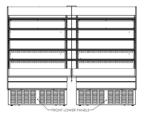
Step #11 Attach lower front cover to holes in base using (4x) black self-tapping screws (p/n V801489).
