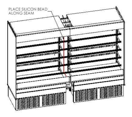
**Step #8** Install the top cover plate using the (6x) self-tapping screws (p/n V801489) in the holes on the top of the machines. Fill in any gaps in the back of the machine with silicone.
