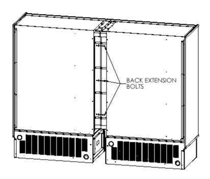
**Step #7** Place approximate 3/8" silicone bead along lower, back and upper seam in the front.
