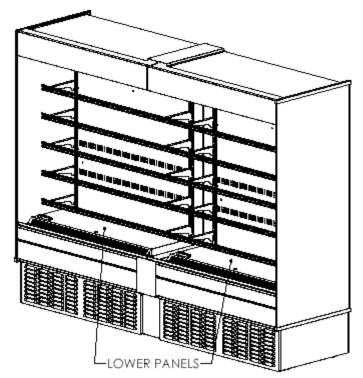
**Step #13** Install top cover in space between the two lower panels. Use (4x) rounded head screws (p/n V802087) to secure and replace the two lower panels.
