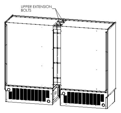
**Step #6** Tighten the remaining bolts, 3 in the back extension and 2 more for the bottom extension.
