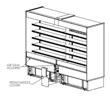
**Step #12** Remove bottom panels by lifting out of the units.
