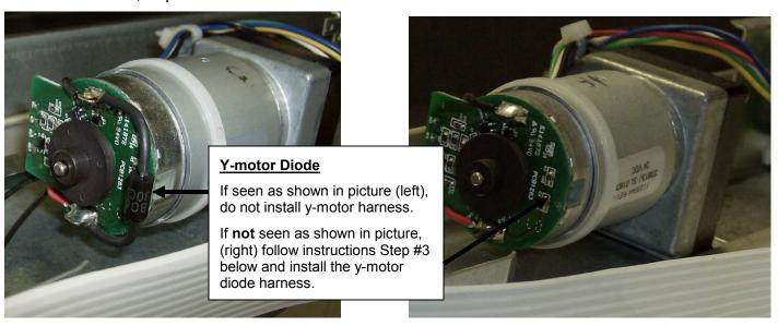
**Step #3 POWER OFF** the machine and install the y-motor diode harness (p/n 1147741) between the top connector on the PC board next to the y-motor and the red and black wire connector coming from the y-motor.
