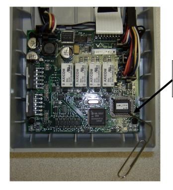
Use a bent paper clip to pry the current EPROM out of the board from the corner
