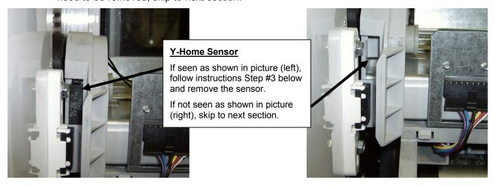
**Step #3** Remove the y-home sensor by removing the (2x) small black screws holding the bracket against the left x-rail end cap. Unplug the harness from the bottom connection located on the PC board and cut the wire tie attaching the harness to the rail.
