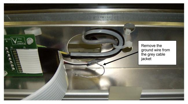
Step #6 Route the grounding harness behind the right motor retainer. Using the wire nut (p/n 1183394), attach the bare end of the grounding harness to the ground wire pulled from the cable jacket in Step #4. Ensure the cable will not interfere with the ribbon cable during movement.
