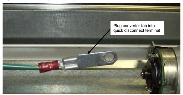
**Step #4** Next, use the self tapping screw (p/n V801489) to attach the other end of the converter tab and the eyelet of the ground wire (p/n 1184099) included in kit to the right side motor retainer bracket next to the PC board.
