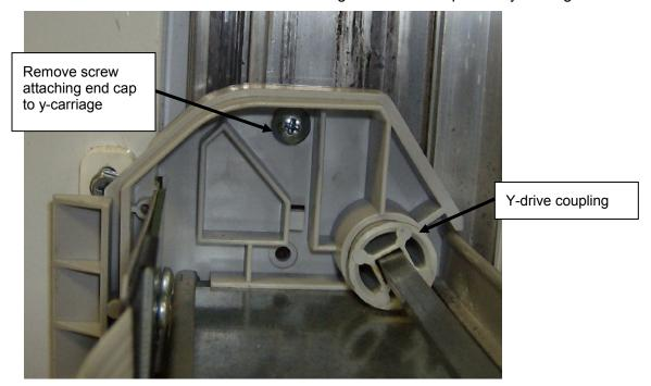
Step #2 Remove the x-rail from the y-carriage by pulling the y-drive coupling away from the end cap. See photo above. Attach the end of the x-rail grounding harness (p/n 1165767) with the eyelet into the x-rail using the existing screw. Route the harness through the rectangle opening in the end cap. Ensure the harness is angled up as shown below to prevent interference. Replace the x-rail into the door tracks and level.
