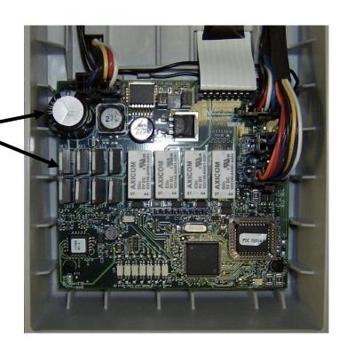
**Step #13** Using a paper clip that has been unfolded, pull out the existing PDC EPROM.
