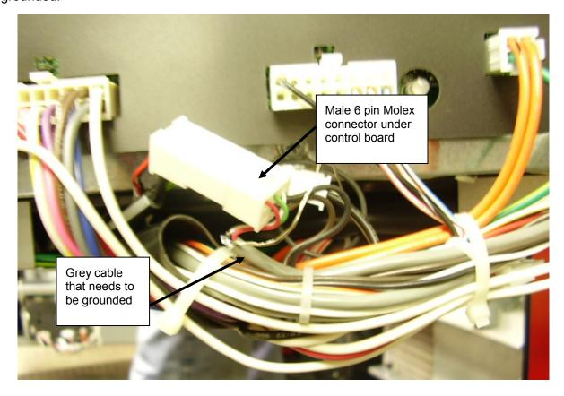
**Note:** For older machines, when the control board is located in the top of the door, the PDC harness is grounded at a stud located in the bottom of the door.
